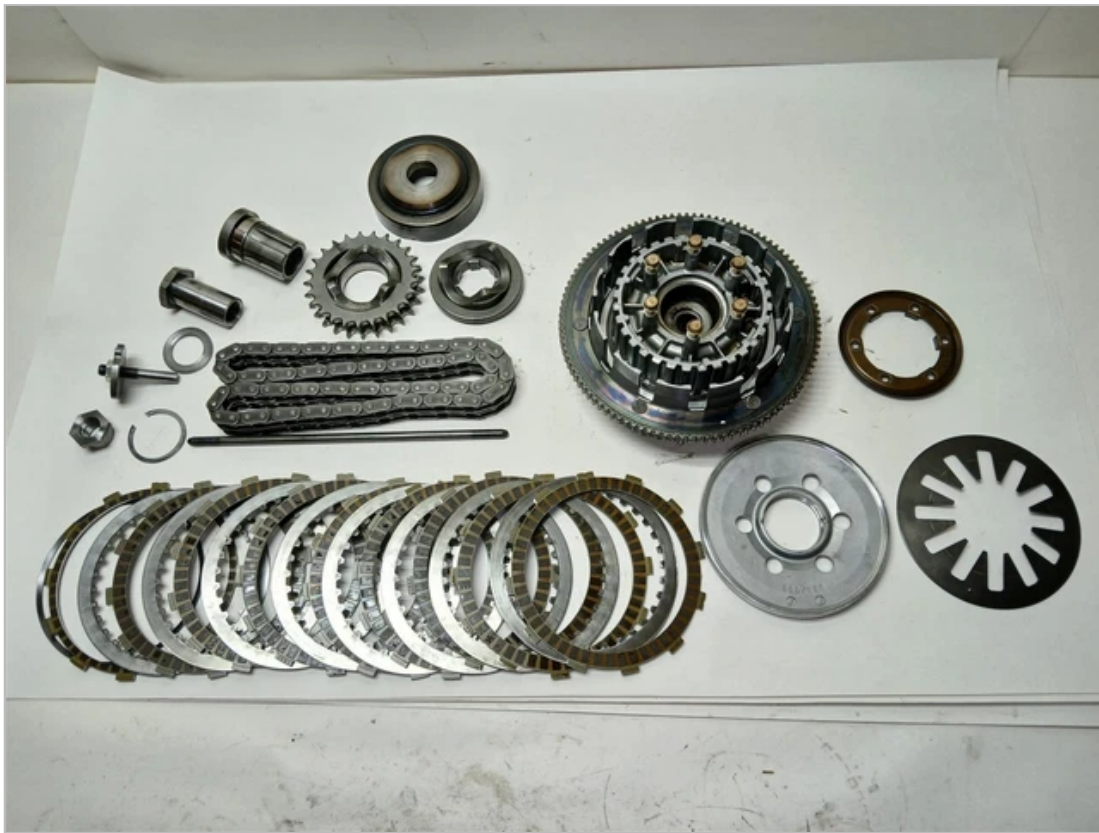
Figure 8. The complete primary drive from a 2002 Softail, laid out in order: compensator parts (upper left), chain, clutch basket with its ring gear (right), and the clutch plate pack fanned out below. Laid out like this, in removal order, reassembly is just this photograph run backwards.
