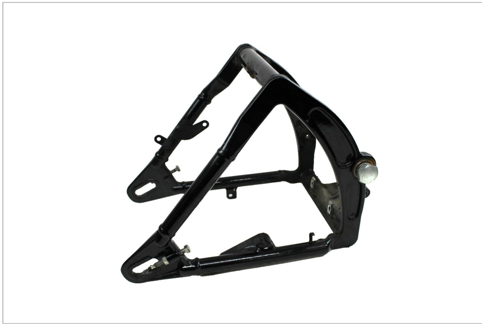
Figure 11. A Softail swingarm off the bike. The wide front cross-tube is the pivot housing — the shaft that runs through it also runs through the transmission case, which is why the arm and the gearbox come apart in the order this section describes.
