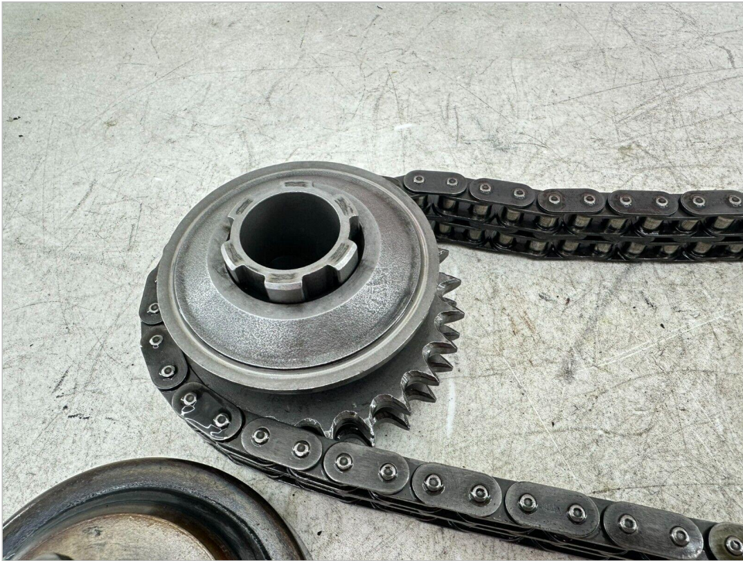
Figure 9. Compensator sprocket and duplex primary chain on the bench. The compensator is the engine's shock absorber: the sprocket drives through a ramped cam and spring pack, which is why its stack order matters and why its nut gets the biggest torque number on the motorcycle.
