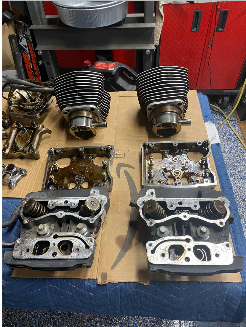
Figure 13. A Twin Cam top end laid out on the bench mid-rebuild — heads, cylinders, and rocker boxes in matched pairs. This is what "organized" looks like: every part with its partner, every fastener with its part, nothing on the floor.
