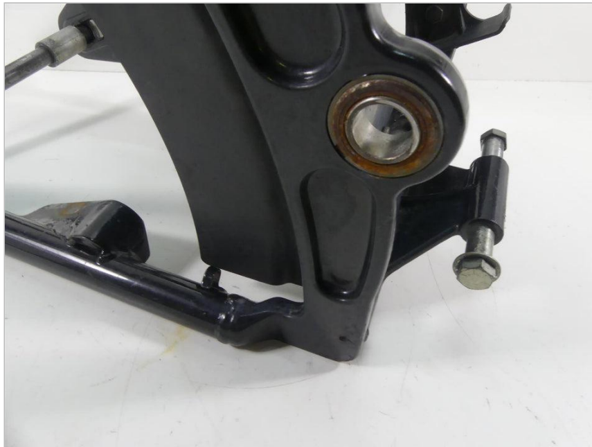
Figure 12. Close-up of a swingarm pivot bearing bore. Clean and inspect these bores and bearings while the arm is out — slop here becomes a weave at highway speed, and you will never have easier access than right now. On reassembly the shaft gets anti-seize so the next man (probably you) isn't fighting your corrosion.
