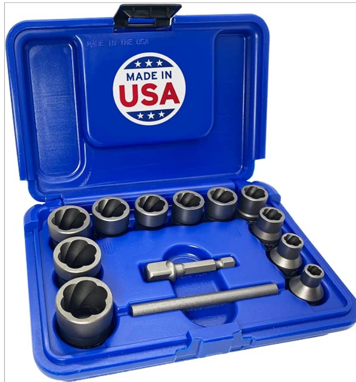
Figure 6. A bolt-extractor ("turbo socket") set. The spiral flutes inside each socket bite into a rounded hex as you turn counterclockwise, gripping harder the more force you apply. Rung 5 lives in this box.
