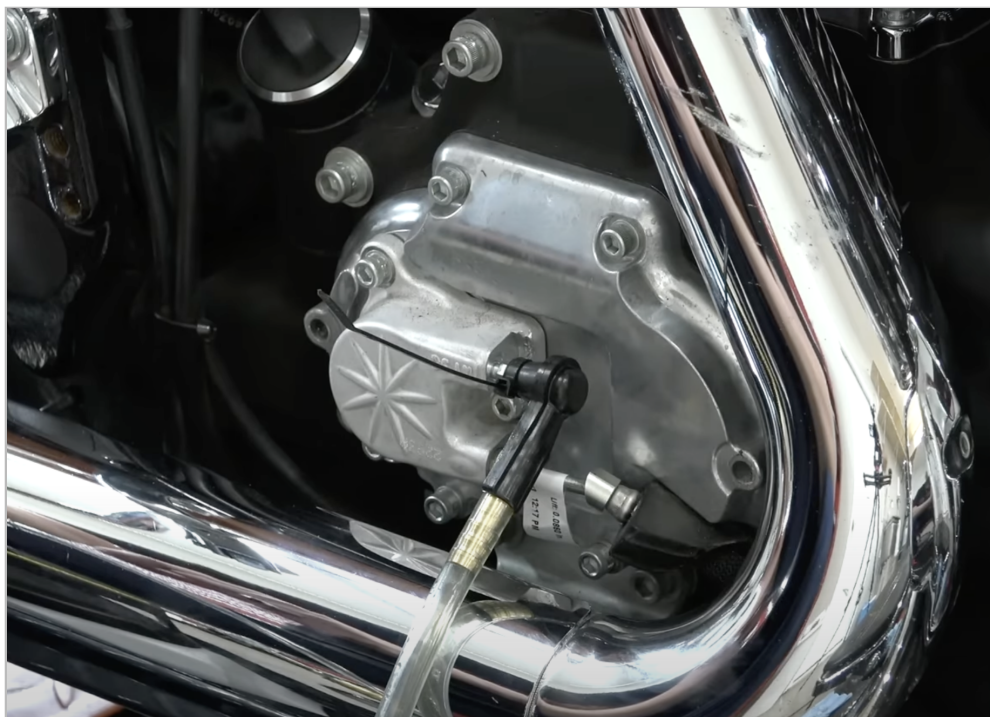
Figure 10. The transmission side (release) cover on the right side of the bike, with the clutch cable coming in from below behind the exhaust. This cover comes off to disconnect the clutch cable, and the whole area is why the exhaust had to come off first.
