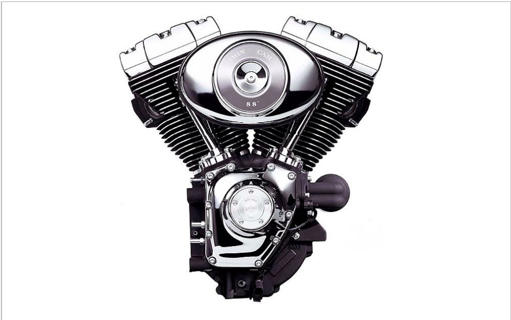
Figure 2. A Twin Cam 88, front view. Learn this silhouette: deep, closely stacked cooling fins, a big round cam cover low on the right side of the cases, and pushrod tubes that run nearly parallel to the cylinders. The factory air-cleaner insert on most of these simply reads "Twin Cam 88."
